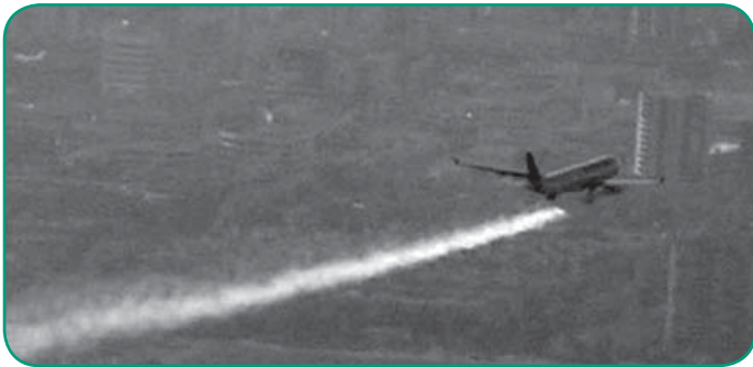
Visible fuel leak from the Airbus A330
