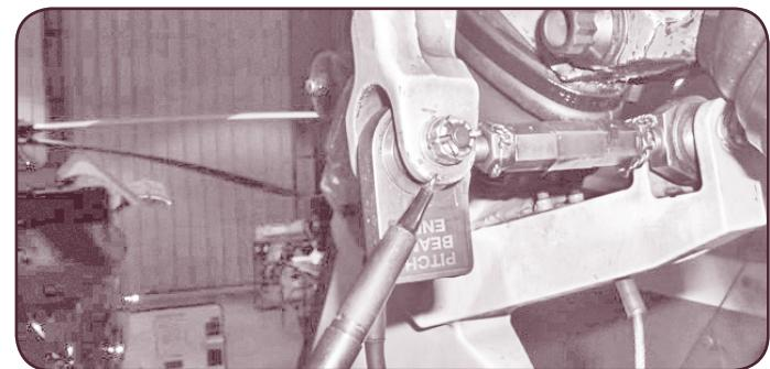
**ENGINES****CF34-3B Missing Nut Engine bleed air port****SDR submitted:**
