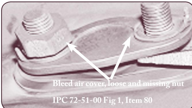
It is unclear whether hot gases were escaping from the loose plate and caused the jet pipe overheat warning or if the nut falling down and contacting the terminal lugs of the sense elements set off the warning.
