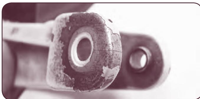
Due to the critical location of the discovered crack, the pitch change beam was replaced and the aircraft was returned to service.
