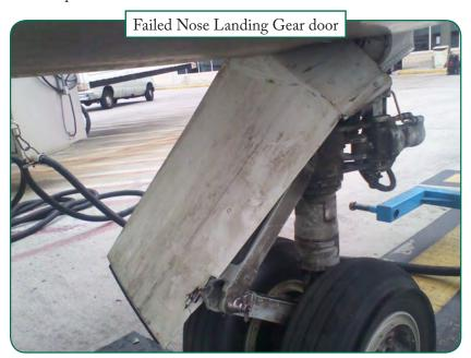
After evaluation of the damages, the door assembly was removed and the aeroplane ferried to a maintenance base for repair. Visual inspection of the NLG area revealed that the aft door had sustained significant damage and
