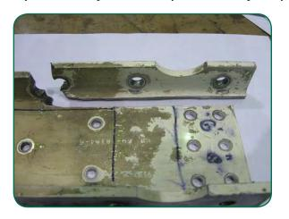
Maintenance was alerted and the aeroplane was towed back to the ramp. Hydraulic fluid was found coming from the belly drains aft of the Nose Landing Gear (NLG) bay. Further maintenance investigation found the NLG lock actuator leaking due to the lock actuator support bracket being cracked.
